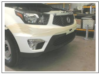
Figure 1: Mask front of vehicle ready to mark.
