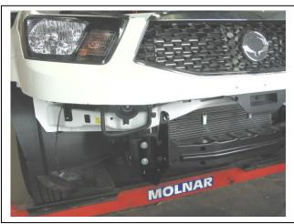
**Figure 1**: Front of completed bumper cut. **NOTE**: retention of centre attachment point.
