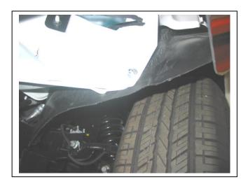
Figure 12: Fitted and trimmed inner guard
