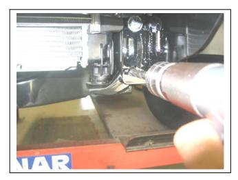
Figure 4: Drill lower mount to 13mm.
