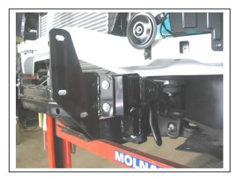
**Figure 3:** Steel mounting bracket installed to chassis rail.
